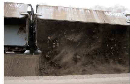
Cleaning from adhering ashes
