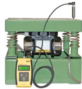
Frequency measurement with VibroScanner at the vibrating table
