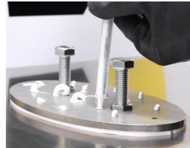
Glue in drill holes
